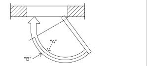
Valve "B" - increases closing speed from maximum openig angle to 20°. Counter-clockwise - increases closing speed.
